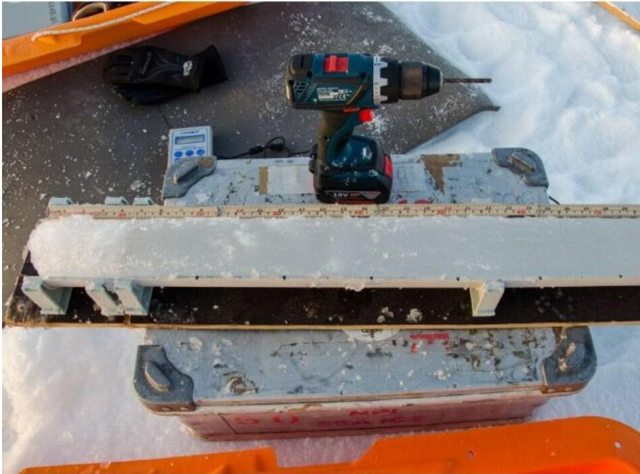
Measuring the length of a sea-ice core, taken on the CAATEX cruise August 2019 near the North Pole. (Photo: Bonnie Raffel)
