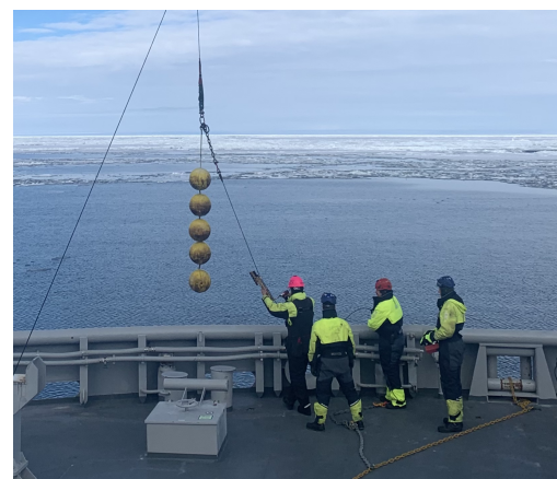
Figure 7: Oceanographic mooring CNRS23, shown here being recovered by KV Svalbard, was localized using active acoustics before being released from its anchor. (Photo: Sofia Vakhutinsky)
