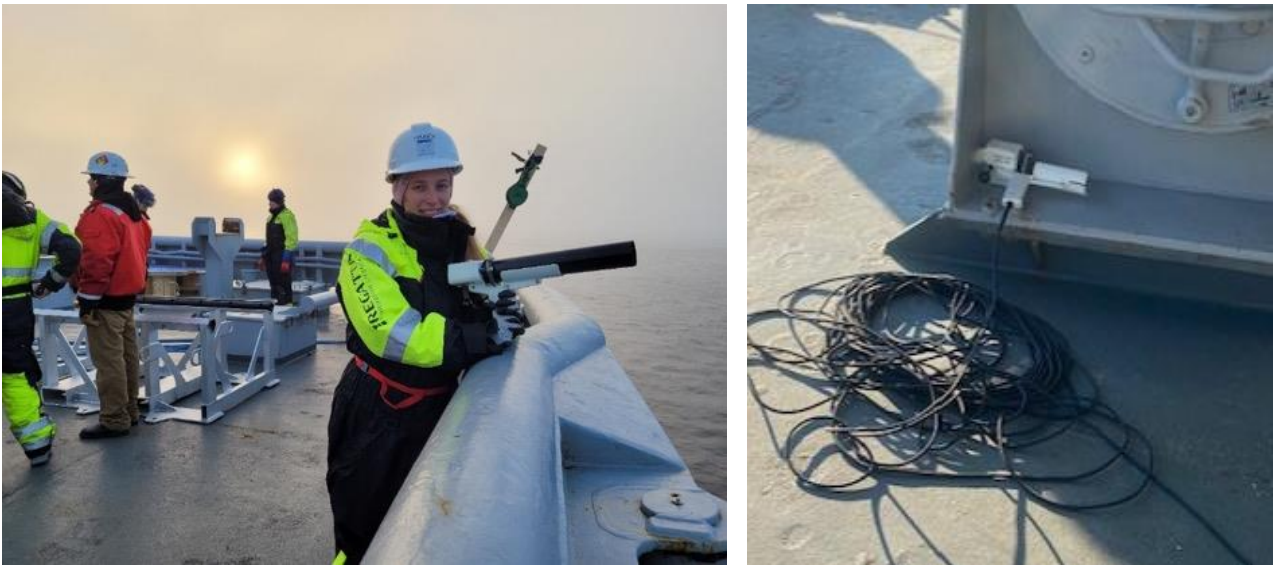
Figure 3.18 Veronica standing ready to launch an XBT at the aft deck (left) and the empty hand-held XBT/XCTD Launcher (right).
