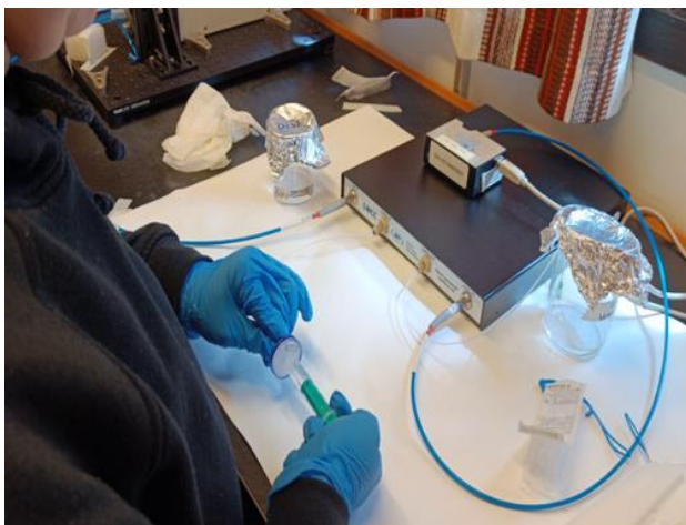
Figure 2.5 CDOM absorption was measured using a Liquid Waveguide Capillary Cell (LWCC)
