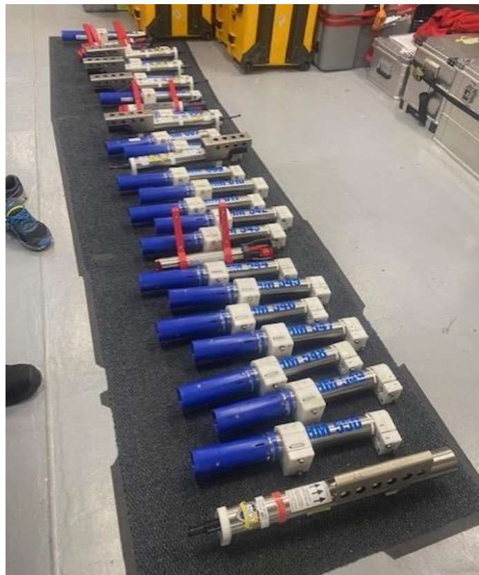
Figure 3.24 Seabirds, hydrophones and RBRs arranged and ready to be attached to the “hairy fairy”.
