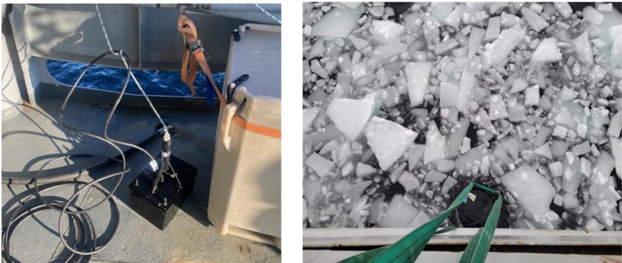
Figure 3.22 The echosounder, Knudsen, used for the bathymetric survey prior to the mooring deployments (left). The tractor tire used to keep drifting ice away from the instrument wire.
