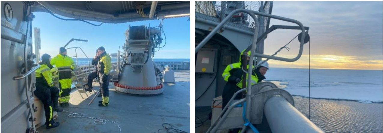
Figure 3.23. The ping team in action on deck (left) with a pulley system for lowering the Knudsen into the water (right).
