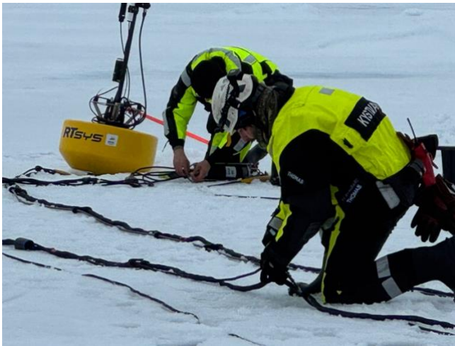
Figure 2. The map in the above panel shows the planned CTD with water bottles (in green) and XCTD stations (in pink) across the Gakkel ridge. The XCTD stations are taken at the locations of the acoustic communication stations. The lower left shows the deployment of the ice tethered buoy with the 100 m long hydrophone array. To the right is a picture of one of the acoustic sources that was used to send communication signals. (Photos by H. Sagen, NERSC, Map by KV Svalbard)
