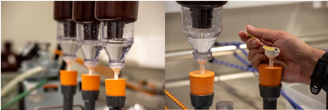
Filtration set-up to collect material for particulate analyses. Photos by Olaf Schneider, Norwegian Polar Institute
